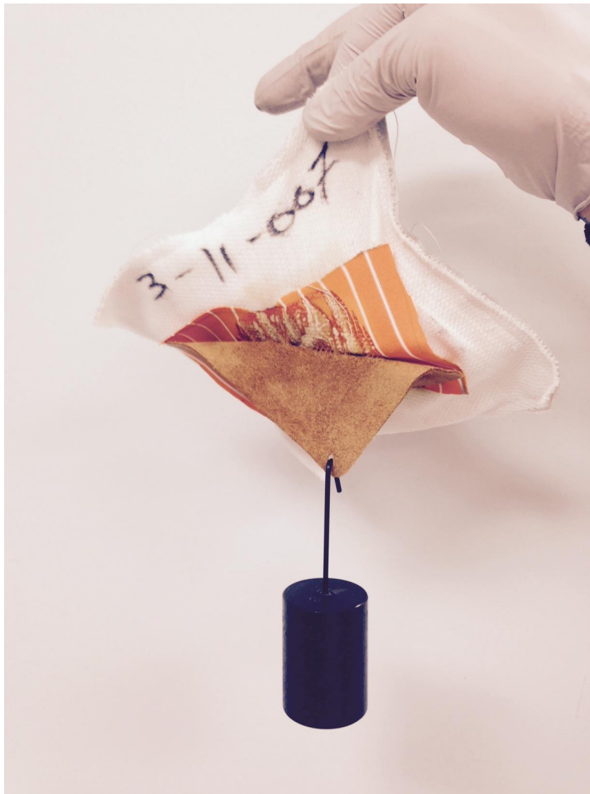
Photo 3, adhesive properties of polyester, 16 seconds exposure
